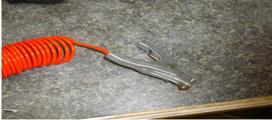
Grounding clip mounts to vacuum base and connect to metal pole
